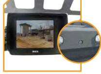
Increase visibility to the rear of the machine with a rear view camera.
