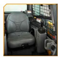
**CHOOSE YOUR RIDE** A high-back, five-way adjustable seat comes as standard. Optional air-ride suspension seat or mechanical suspension seat provide enhanced comfort.
